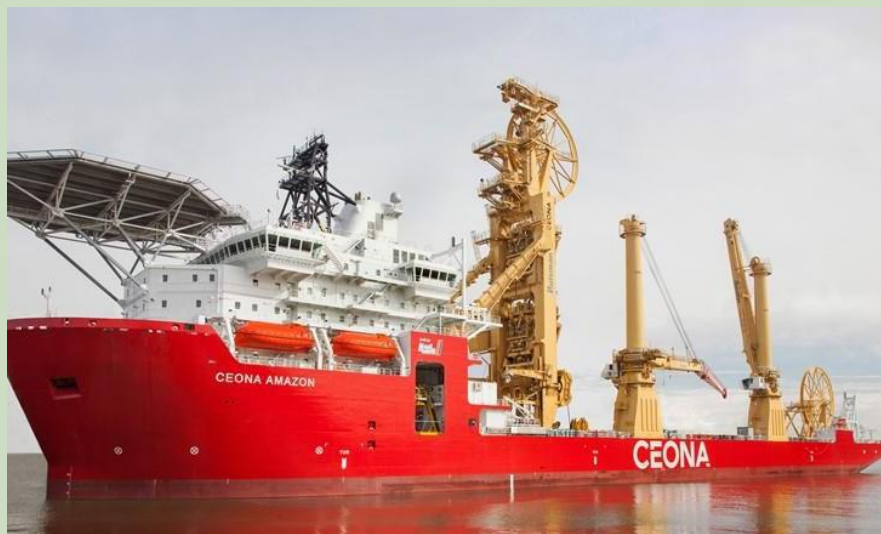
2 x 400 t heavy lift system (to 3000 m depth)
